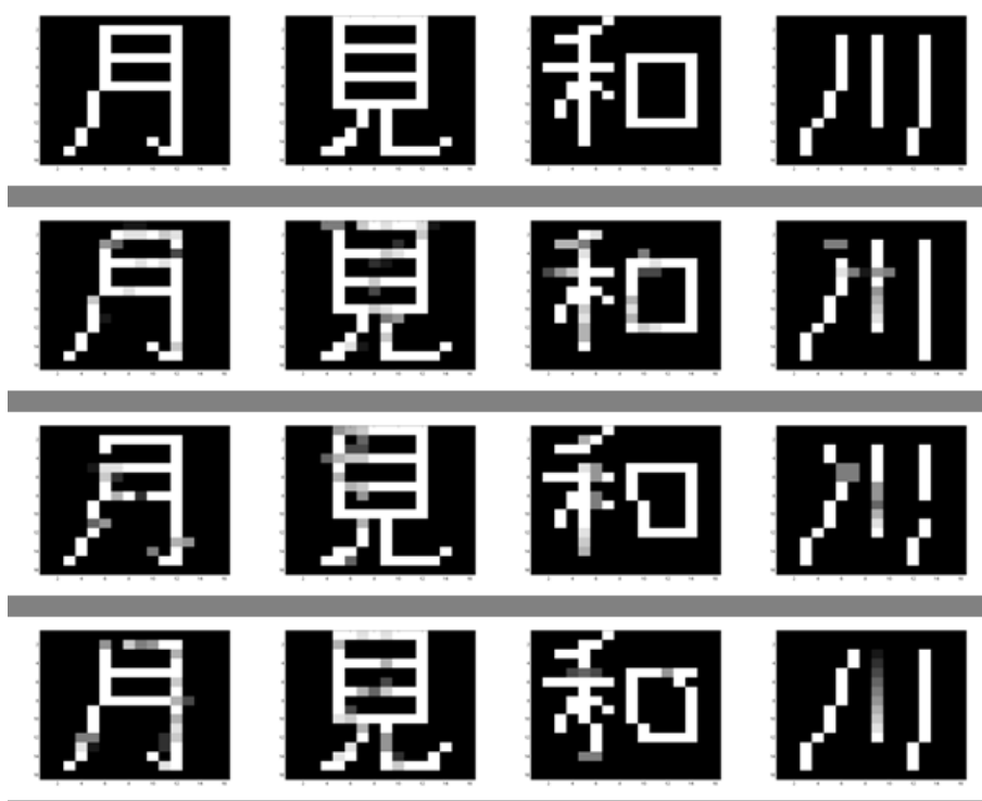
Figure 2.15: A 256 - 4 - 2 FFNN was trained to distinguish between the four kanji signs in the first row. The resulting FFNN produced the correct output for each kanji sign, including the 12 noisy versions shown in the bottom three rows.
