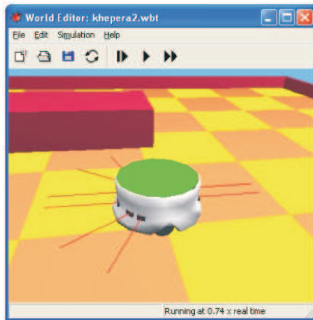
Figure 3.26: A screenshot from a Webots TM simulation of a Khepera II robot. Reproduced with kind permission of Dr. O. Michel, Cyberbotics.
