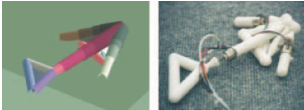
Figure 3.25: A crawling robot evolved by Lipson and Pollack [67]. The left panel shows the simulated robot, and the right panel shows the corresponding physical robot. Reproduced with kind permission of Dr. H. Lipson.
