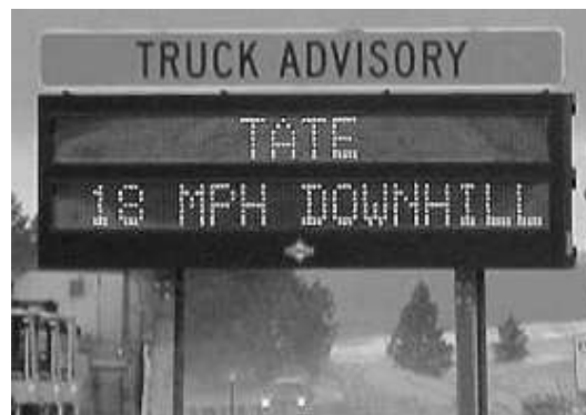
Figure 4.4: Recommended downhill cruising speed that is custom made to the driver. Emigrant hill, Interstate 84, Oregon, USA. With permission from: Oregon Department of Transportation Traffic Engineering & Operations, ITS Unit.
