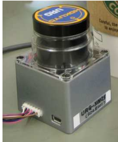
Figure 7.3: A laser range finder (URG-X002S) manufactured by Hokuyo. Photo by the author.
