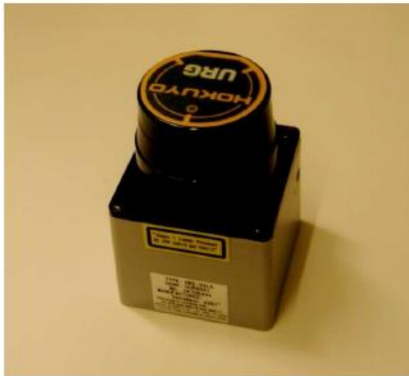
Figure 1.8: Left panel: A Hokuyo URL-04LX laser range finder. Right panel: A typical reading, showing the distance to the nearest object in various directions. The pink rays indicate directions in which no detection is made. The maximum range of the sensor is 4 m.
