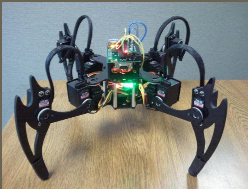
Quadruped robot with Arduino microcontroller
